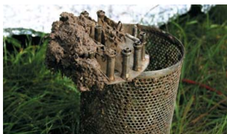
SPMD for passive sampling of lipophilic organic compounds after three weeks of exposure in the River Elbe close to Pardubice (Czech Republic)
