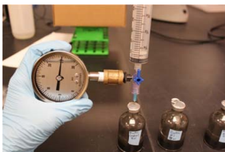
Figure I.5-2. Monitoring Pressure Within Reactors.
